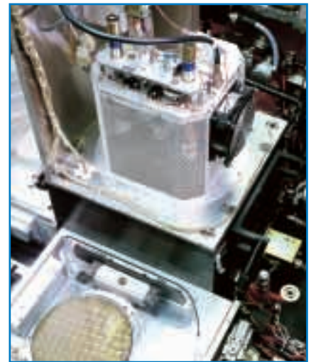
The AE Sparcle line of pulsing units combine with a separate DC power supply to provide flexible pulsing
