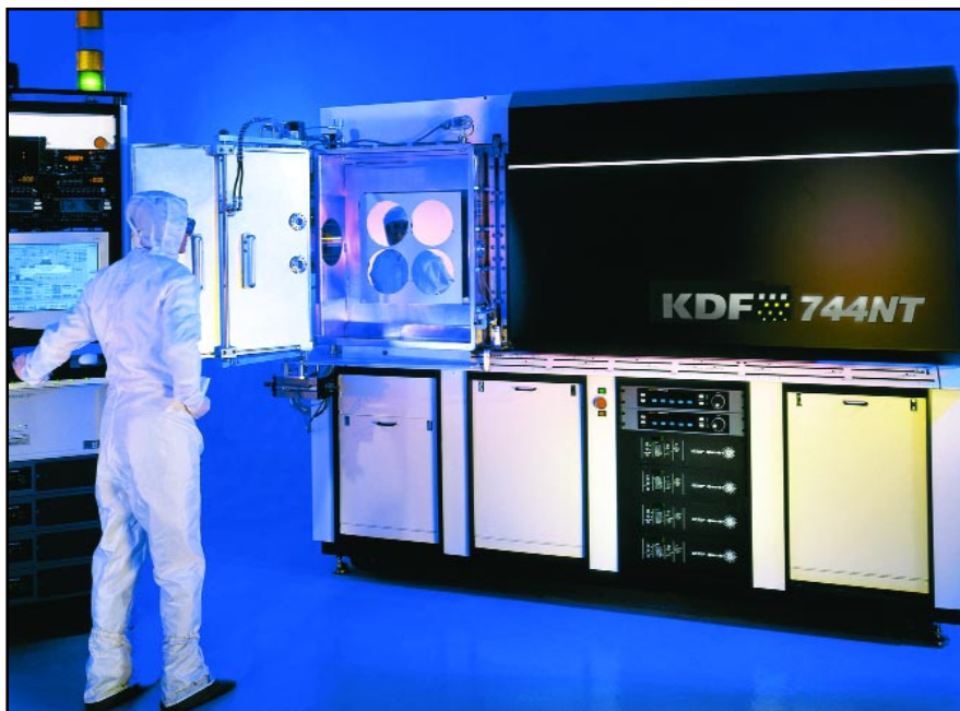
Using standard components and a switching power supply, a New Jersey company has developed a DC reactive sputtering technique that promises to greatly reduce the time required to deposit dielectric films. The KDF 744 system will target the organic LED market.
