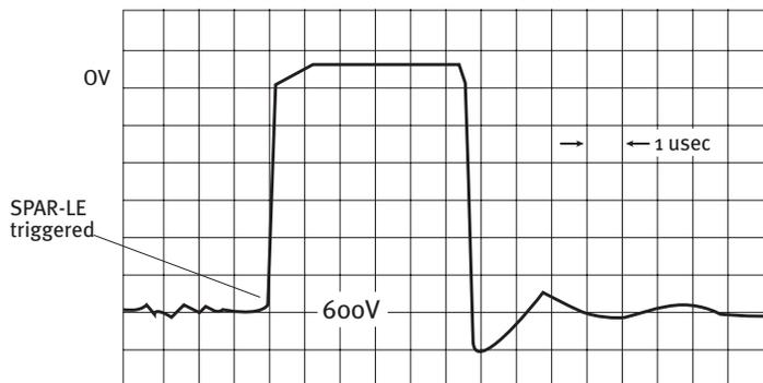
Figure 4. SPARC-LE® waveforms, self run mode
