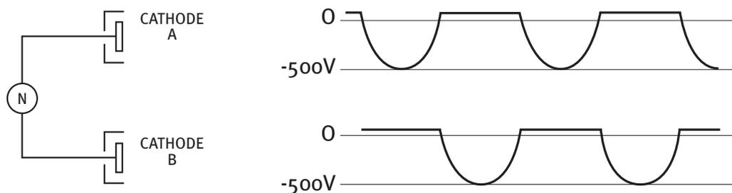
Figure 6. Dual-cathode system, idealized waveforms
