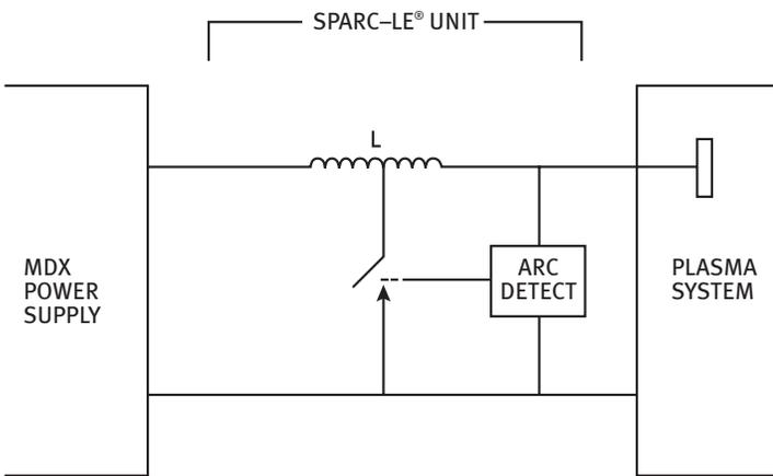
Figure 2. SPARC-LE® unit simplified schematic
