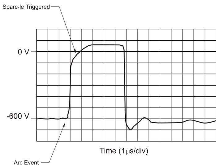
Figure 5. SPARC-LE® waveforms, arc triggered
