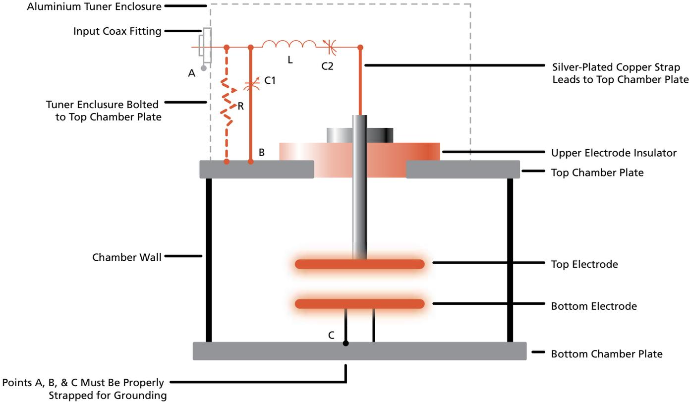
Figure 2. Tuner-to-chamber installation (tuner is mounted directly to the top plate of the chamber)
