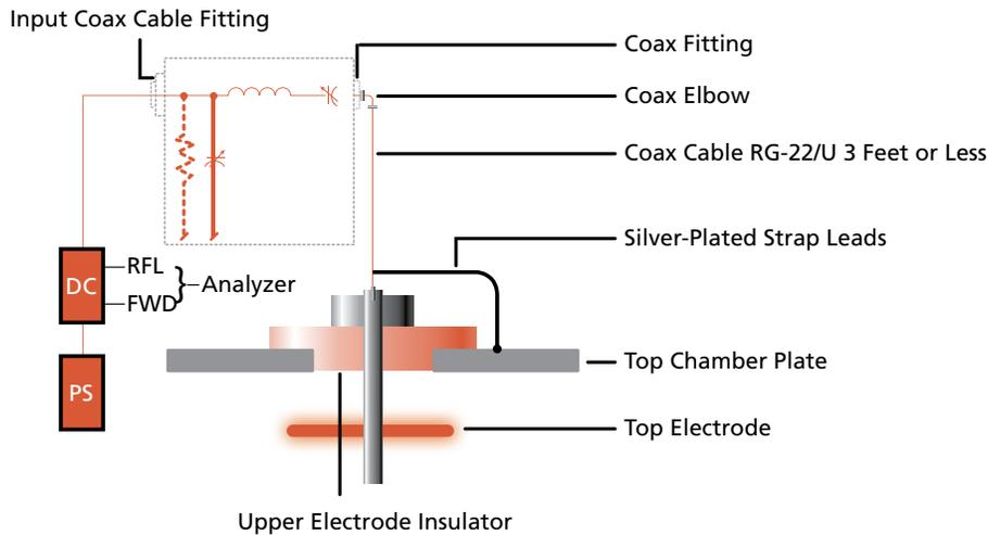
Figure 3. Chamber installation (using coaxial cable from tuner output to chamber plates) and calibration
