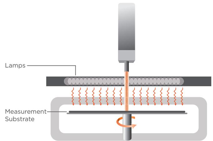
Measurement in Lamp Heated Reactor
