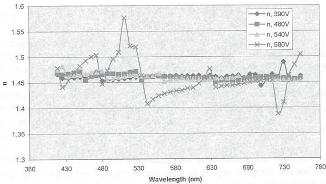
Figure 5: Index of Refraction versus Sputter Voltage
