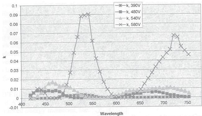
Figure 6: Coefficient of Extinction versus Sputter Voltage
