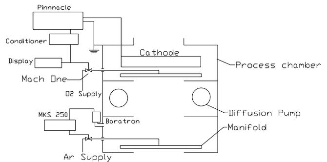
Figure 2: Process Chamber Setup
