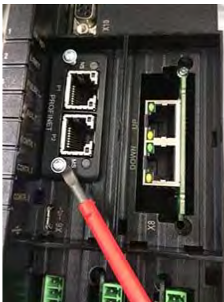
Figure 6. Anybus module removal
