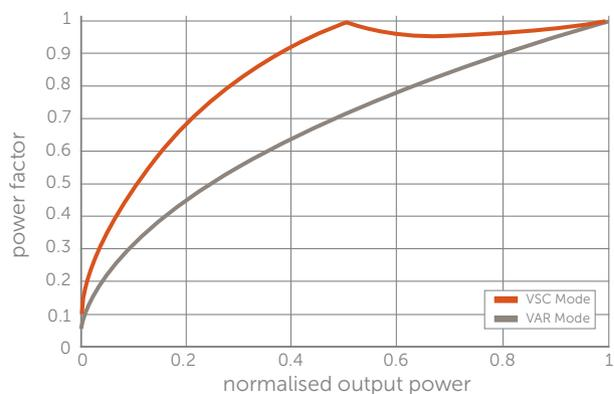
**Illustration 6: Power factor in accordance to output effective power (modulation) of 2-stage VSC connection**
