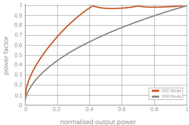
Illustration 2: Power factor in accordance to output effective power (modulation) of 3-stage VSC connection
