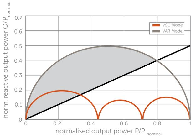
**Illustration 3: Reactive power as function of the released effective power at 3-stage VSC connection**
