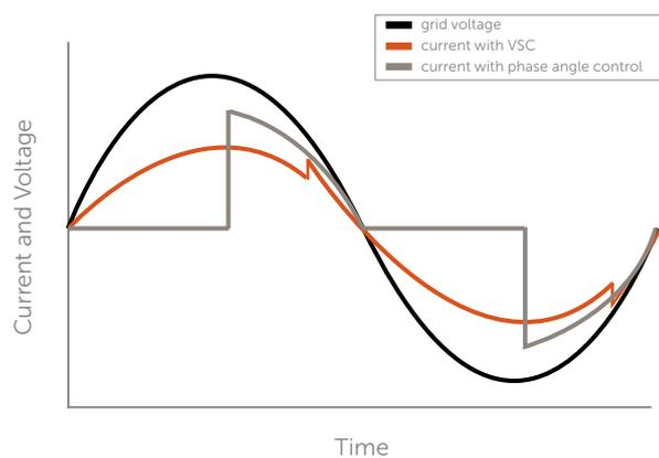
**Illustration 8: Comparison of phase angle firing (VAR) and VSC (Voltage-Sequence Control) with same effective current value**
