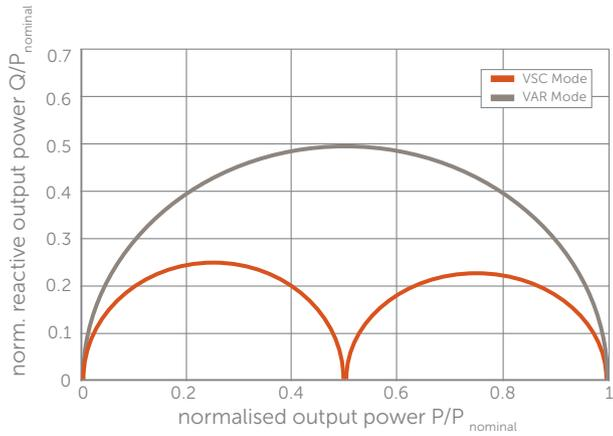
**Illustration 7: Reactive power as function of released effective power at 2-stage VSC connection**
