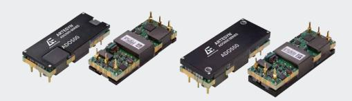
ADO500/550 series eighth-brick isolated DC-DC converters produce a single fully regulated 10 V output. Rated at 500/550 watts, these converters can deliver up to 55 amps output current and have no minimum load requirement. They have an input voltage range of 45 to 56 V and are primarily designed for use with standard 48 V supplies in computing and server applications, as well as regulated 48V supplies in communications equipment.
