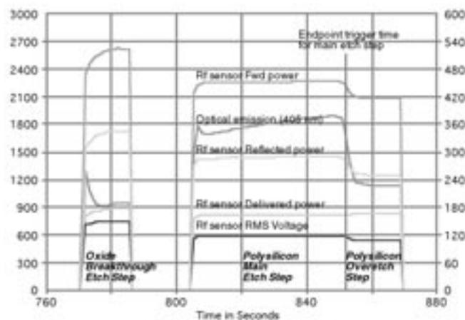
**Figure 2. A set of waveforms gathered during the etch of a polysilicon wafer on a Lam 490 AutoEtch. Shown are a portion of the RF parameters available, plotted along with a standard optical emission parameter for reference**
