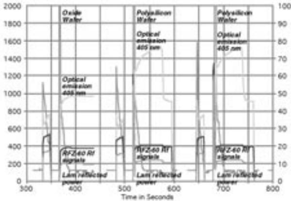
Figure 3. Polysilicon etch on a Lam 490. This was an attempt to recreate a recurring problem, with the thought that it was due to an incomplete oxide strip after POC13 deposition. This test was not successful, as residual oxide was not the problem mechanism. But, the oxide wafer gave an optical trace signature similar to that seen during previous problem etches.
