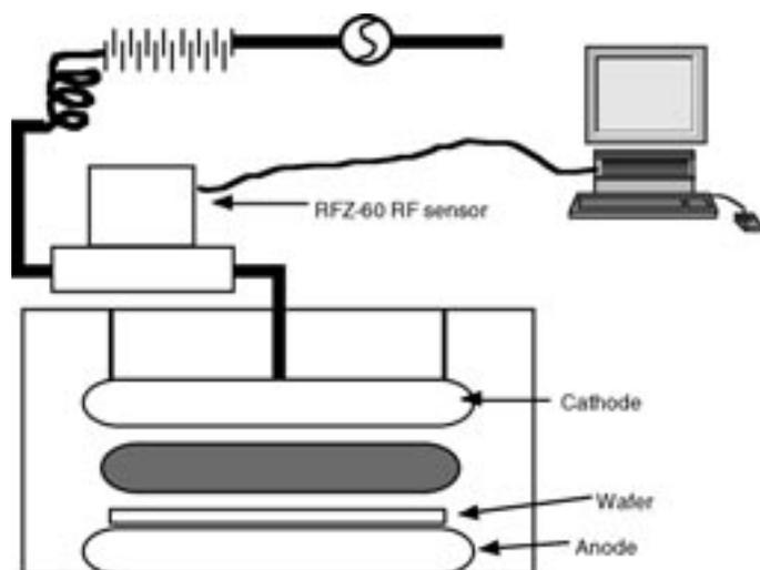
**Figure 1. The positioning of the Advanced Energy RFZ-60 RF sensor in the Lam 490 etching tool**
