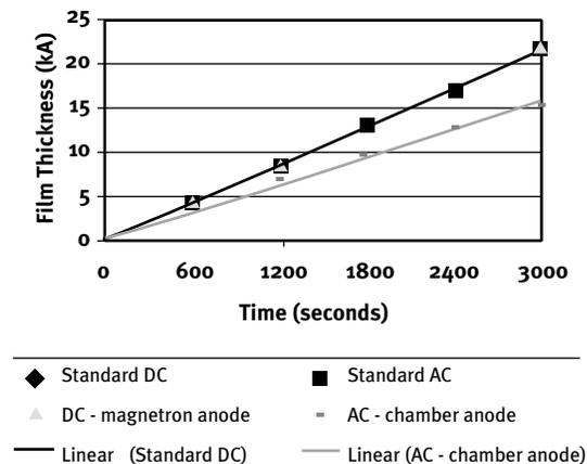
**Figure 3. Substrate deposition rates at 2.5 kW; values of 7.2 and 5.3 A/sec calculated for DC-CA and AC-CA, respectively**
