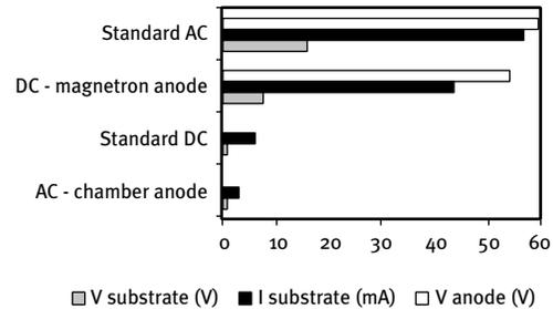
**Figure 4. Self-bias voltages and ion currents on the substrate and anode**
