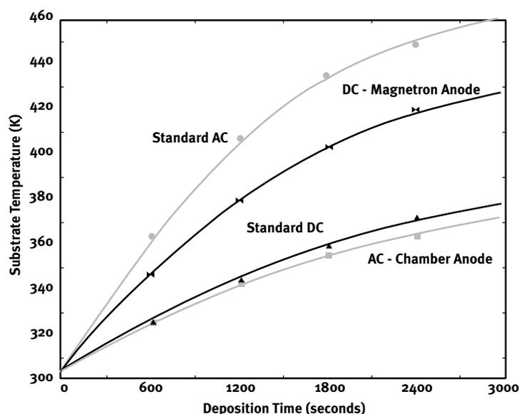
Figure 2. Temperature rise profiles for tested configurations; points indicate actual measurements and lines represent the best empirical fit of the energy balance (see Equation 1) with  $\epsilon = 0.20$
