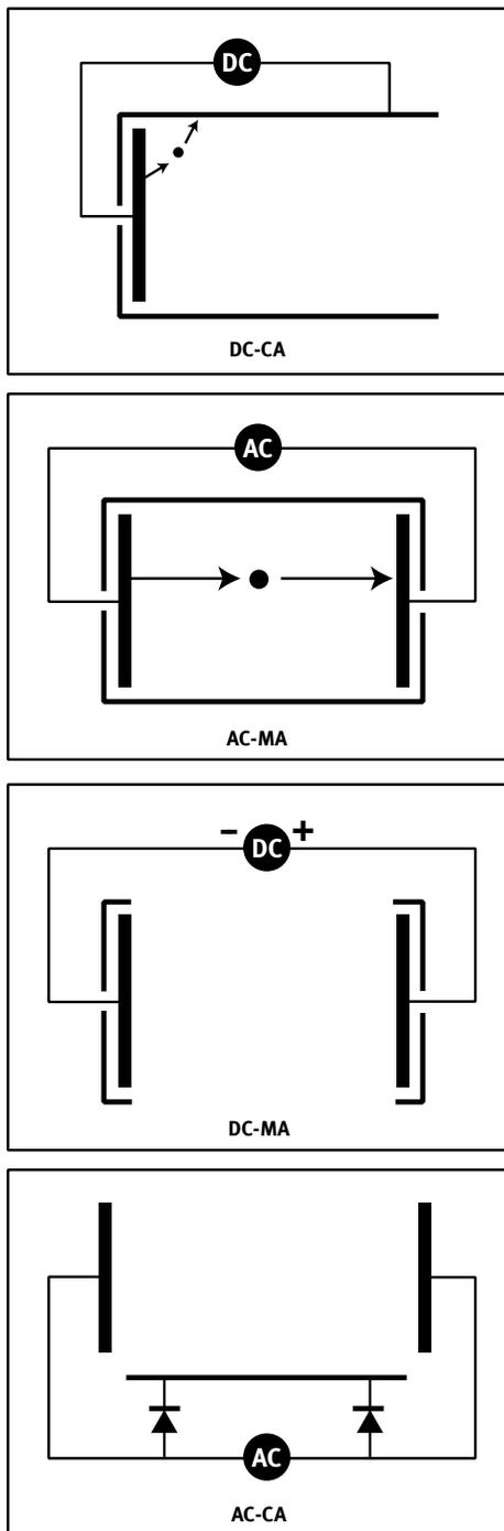
Figure 1. Tested configurations, first two letters indicate method of power delivery while the last specify the system anode:
