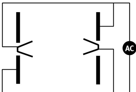
Figure 5. Crossed anode configuration utilizing center anode posts
