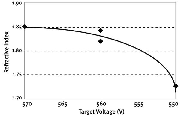
Figure 8. Refractive index of aluminum oxide thin films made under different voltages
