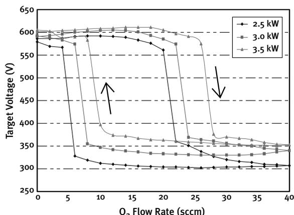
Figure 3. Hysteresis curve with open loop
