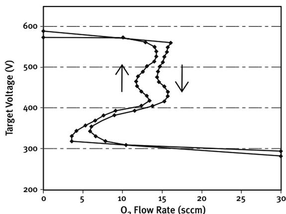
Figure 4. Hysteresis curve with closed loop control at 2.5 kW output
