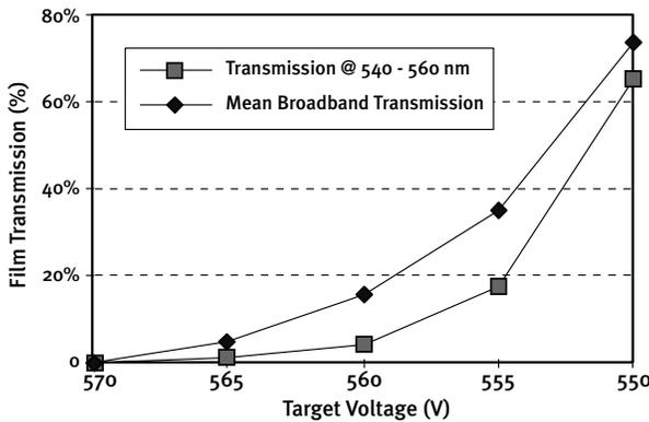
Figure 7. Film transmission at different target voltages under 3.0 kW output power
