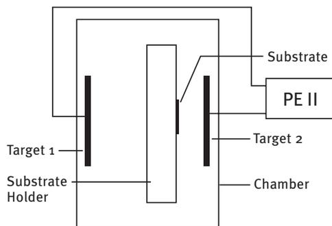
**Figure 2. The chamber configuration of the experimental system**
