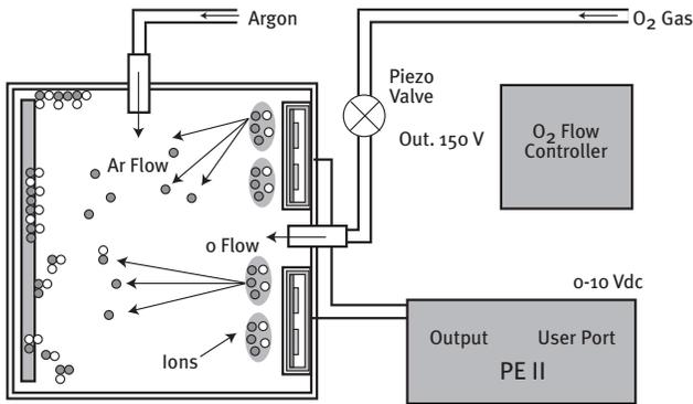
**Figure 1. A typical chamber configuration of closed loop controlled dual magnetron reactive sputtering**
