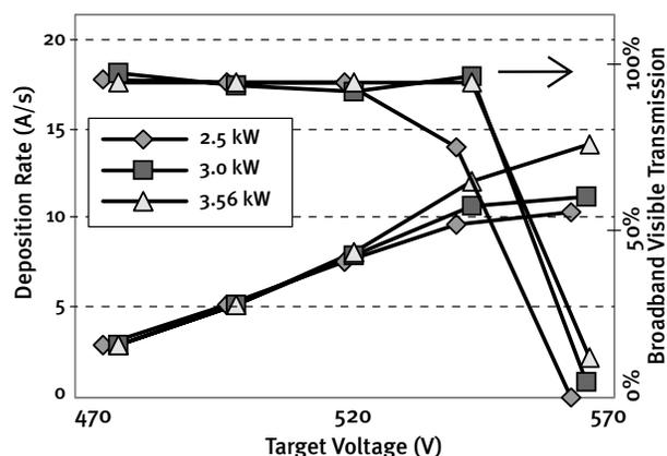
Figure 6. Reactively sputtered aluminum oxide deposition rate and film transmission
