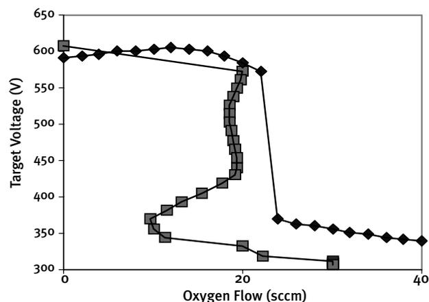
Figure 5.  $Al_2O_3$  target voltage hysteresis curves of open loop versus closed loop
