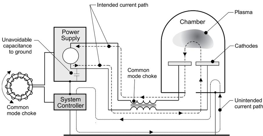
figure 13 common-mode choke
