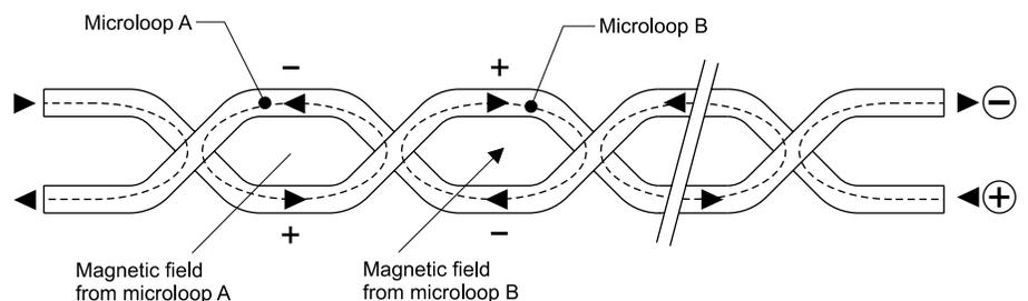
figure 9 twisted-pair cable
