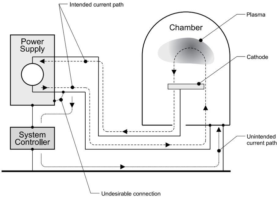
figure 11 multiple current paths in dc power system
