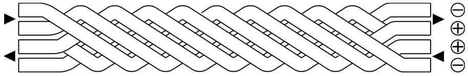
figure 10 twisted-quad cable
