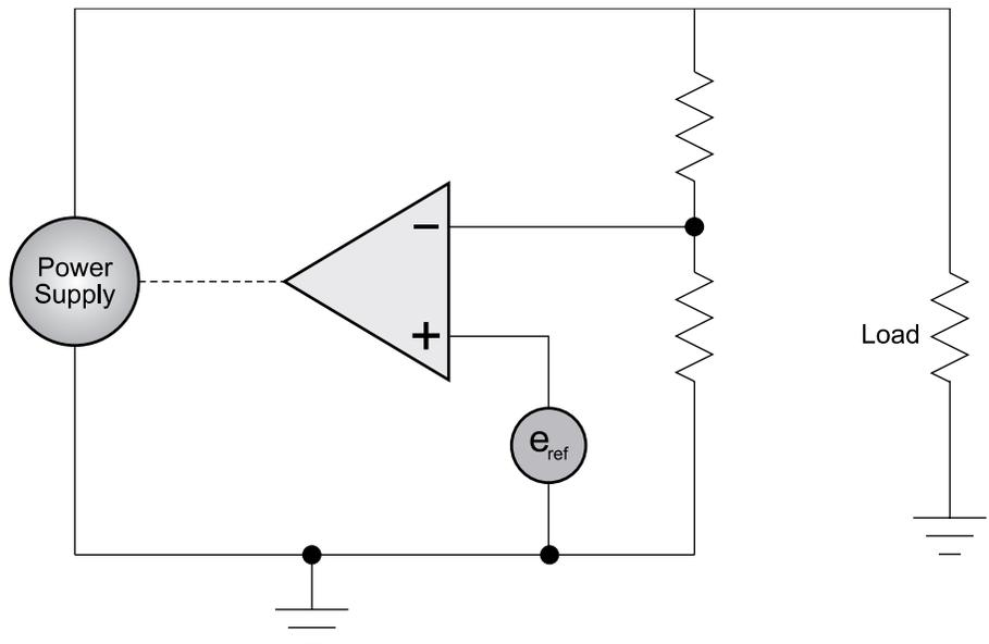
figure 1 regulated power supply (supposed circuit)
