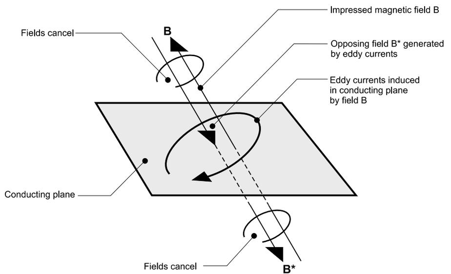
figure 5 time-varying magnetic field inducing currents
