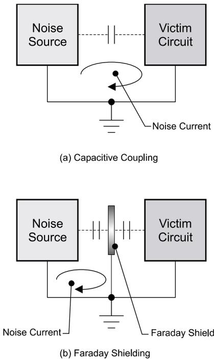
figure 4 capacitive coupling and faraday shielding
