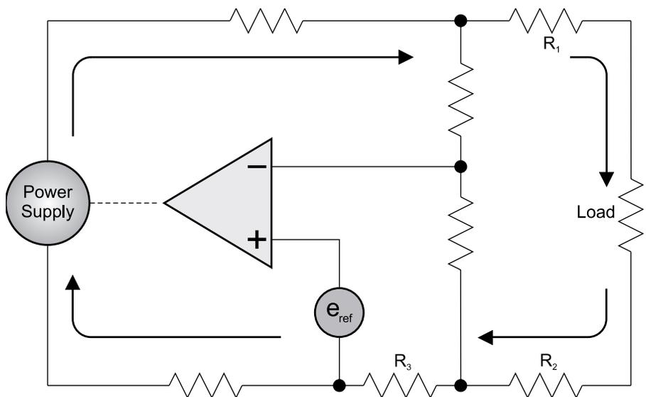
figure 2 regulated power supply (actual circuit)
