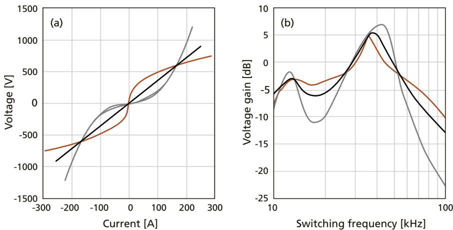
Figure 3 a) Load characteristics and b) gain curves for each respective load
