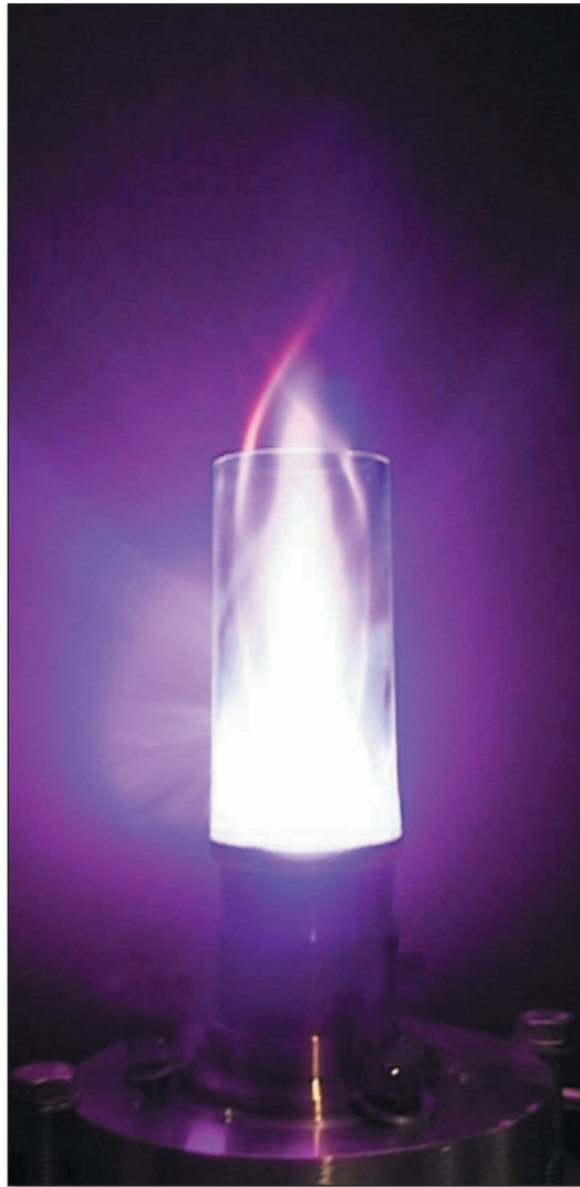
Figure 4 The plasma source in the Litmas Red™ atmospheric pressure abatement system, with its protective covers removed. The plasma plume shown is formed from 100% nitrogen, using only electricity as fuel. The diameter of the plasma region is 5 cm
