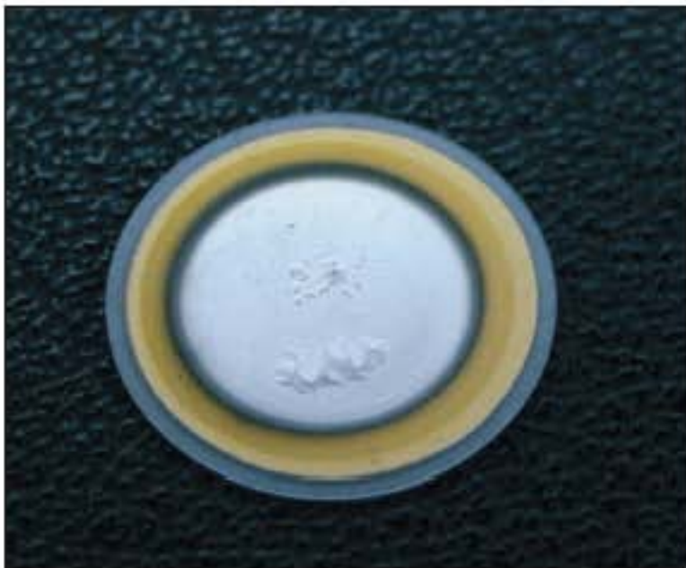
Photo of a substrate showing meteor defects caused by arcing
