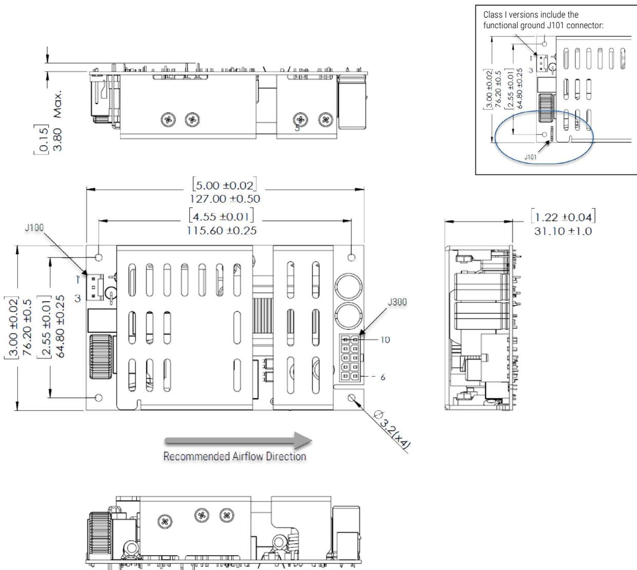
Note 1 - Dimensions: W: 3.0" x L: 5.0" x H: 1.37" (W: 76.2 mm x L:127 mm x H: 34.9 mm).
