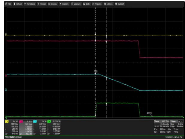
Figure 14: LCM600L DCOK Signal Turn-off Delay - Vin = 100Vac Load: Io = 2A (12V), I SB = 0A (5V) Ch 1: AC Mains Ch 2: ACOK Ch 3: Vo Ch 4: DCOK
