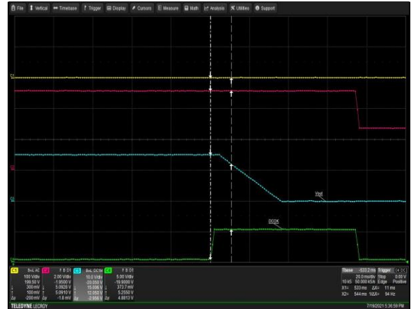
Figure 29: LCM600N DCOK Signal Turn-off Delay - Vin = 100Vac Load: Io = 2A (15V), I SB = 0A (5V) Ch 1: AC Mains Ch 2: ACOK Ch 3: Vo Ch 4: DCOK
