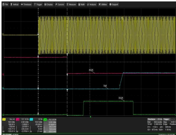
Figure 11: LCM600L ACOK Signal Turn-on Delay - Vin = 100Vac Load: Io = 2A (12V), I SB = 0A (5V) Ch 1: AC Mains Ch 2: ACOK Ch 3: Vo Ch 4: DCOK
