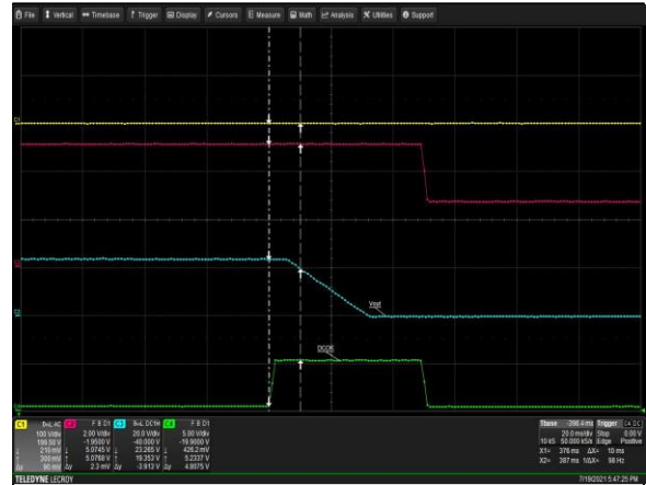
Figure 44: LCM600Q DCOK Signal Turn-off Delay - Vin = 100Vac Load: Io = 2A (24V), I SB = 0A (5V) Ch 1: AC Mains Ch 2: ACOK Ch 3: Vo Ch 4: DCOK
