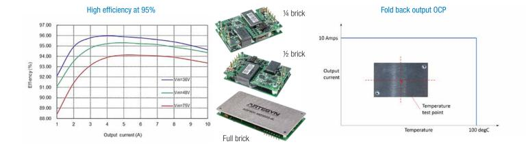
Artesyn's DCDC converters address these application demands. All of the DCDC converters possess high conversion efficiency in the region of 95% and their calculated reliability exceeds 1.5 million hours. Additionally, the current limiting characteristic of Artesyn's DCDC modules exhibits an auto-recovery over current protection mode of operation even if the unit gets overloaded.
