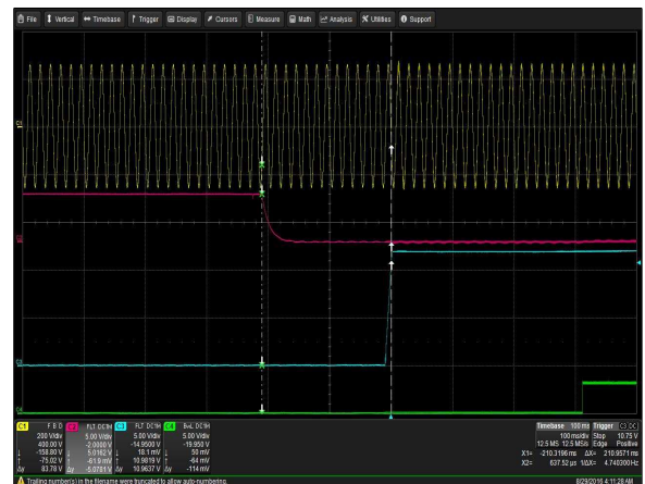
Figure 4: DS2000SPE-3 Turn-on Delay via PS_ON Vin = 180Vac Load: I_O = 160.5A I_{SB} = 3.5A Ch 1: AC Mains Ch 2: PS_ON_L Ch 3: V_O Ch 4: PWOK
