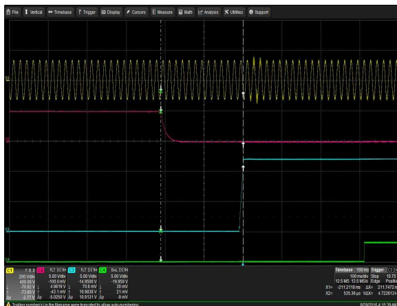
Figure 3: DS2000SPE-3 Turn-on Delay via PS_ON_L Vin = 90Vac Load: I_O = 78.52A I_{SB} = 3.5A Ch 1: AC Mains Ch 2: PS_ON_L Ch 3: V_O Ch 4: PWOK
