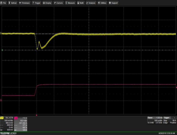
Figure 13: DS2000SPE-3 Transient Response - V_O Deviation 25% to 75% load change 0.5A/uS slew rate V_{in} = 230V_{ac} Ch 1: V_O Ch 2: I_O
