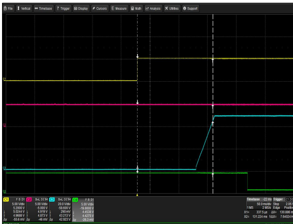
Figure 23: iMP1-5W0-00-A Turn-on Delay via Global inhibit Vin = 90Vac Load: I_o = 25A I_{sb} = 1A Ch 1: Global inhibit Ch 2: V_{sb} Ch 3: V_o Ch 4: Global DCOK
