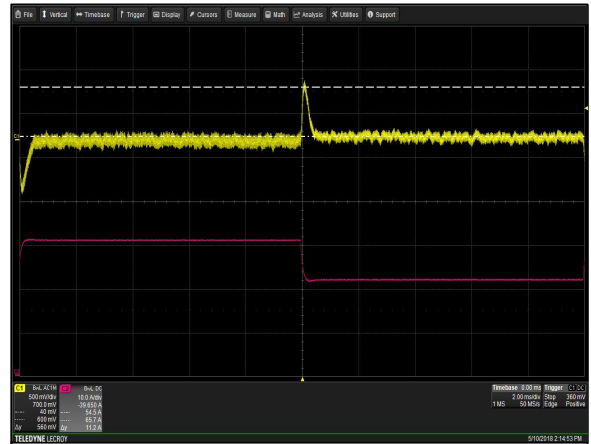
Figure 49: iMP1-5W0-00-A Transient Response - V O Deviation Vin = 230Vac 100% to 70% load change, 1A/µs slew rate Ch 1: V O Ch 2: I O
