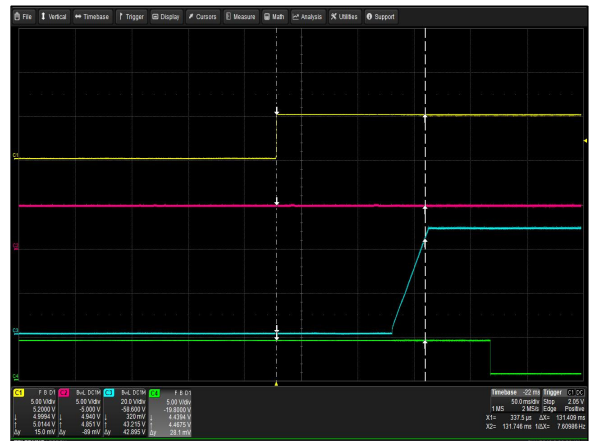
Figure 24: iMP1-5W0-00-A Turn-on Delay via Global inhibit Vin = 180Vac Load: I_o = 31.25A I_{sb} = 1A Ch 1: Global inhibit Ch 2: V_{sb} Ch 3: V_o Ch 4: Global DCOK
