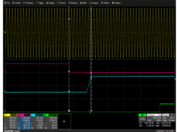
Figure 2: CSU2400AT-3-100 Turn-On Delay via PS_ON Vin = 264Vac Load: I_o = 196.7A I_{SB} = 3.5A Ch 1: AC Mains Ch 2: PS_ON Ch 3: V_o Ch 4: PWOK
