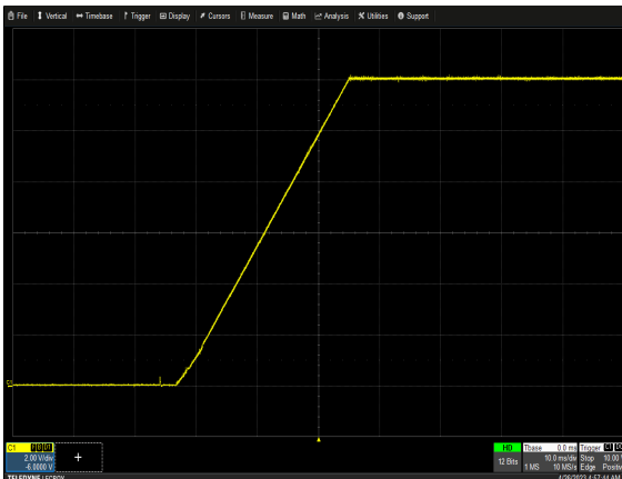
Figure 9: CSU2400AT-3-100 Output Voltage Startup Characteristic V_{in} = 180V_{ac} Load: I_o = 196.7A I_{SB} = 3.5A Ch 1: V_o
