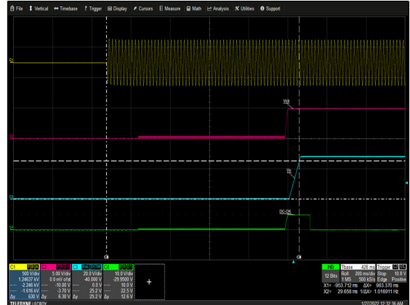
Figure 2: LCC1200-28U-9P Turn-on delay via AC mains Vin = 264Vac Load: Io = 42.9A (28V), I SB = 1.5A (5V) Ch 1: AC Mains Ch 2: V SB Ch 3: V O CH 4: G_DCOK_C
