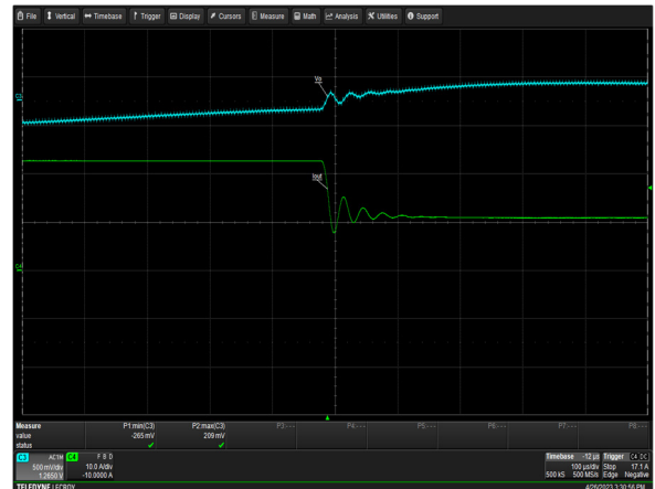
Figure 22: LCC1200-48U-9P Transient Response - Vo Deviation 100% to 50% load change (1KHz) 1A/uS slew rate Vin = 230Vac Ch 1: V O Ch 2: I O
