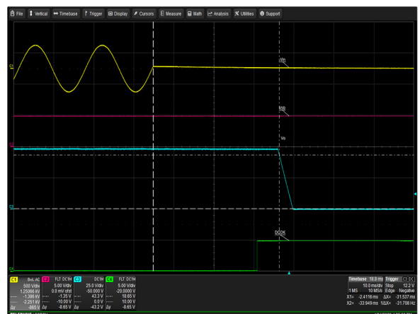
Figure 18: LCC1200-48U-9P Hold-up Time Vin = 264Vac Load: Io = 25A (48V), I SB = 1.5A (5V) Ch 1: AC Mains Ch 2: V SB Ch 3: V O CH 4: G_DCOK_C
