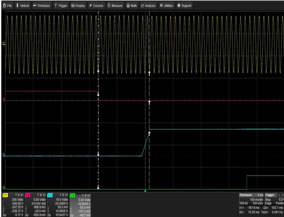
Figure 14: CSU2400AP-3-111 Turn-On Delay via PSON Vin = 180Vac Load: I O = 196.7A I SB = 3.5A Ch 1: AC Mains Ch 2: PSON Ch 3: V O Ch 4: PWOK
