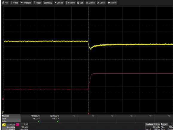
Figure 22: CSU2400AP-3-111 Transient Response - V O Deviation 40% to 100% load change 0.5A/μs slew rate Vin = 230Vac Ch 1: V O Ch 2: I O
