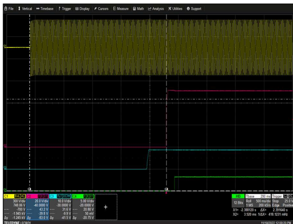
Figure 3: AIF11BAC-01N Turn-On Delay via AC Mains Vin = 264Vac Load: I O = 10.5A I SB = 0.25A Ch 1: AC Mains Ch 2: V O Ch 3: V SB Ch 4: PSU-GOOD
