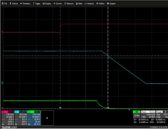
Figure 7: AIF11BAC-01N Turn Off Characteristic via PS_ON Vin = 230Vac Load: I o = 10.5A I SB = 0.25A Ch 2: PSU ENABLE Ch 3: V O Ch 4: PSU-GOOD
