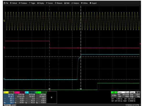
Figure 2: AIF11BAC-01N Turn-On Delay via PSON Vin = 90Vac Load: I O = 10.5A I SB = 0.25A Ch 1: AC Mains Ch 2: PSU ENABLE Ch 3: V O Ch 4: PSU-GOOD
