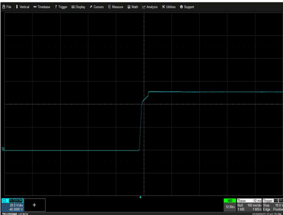
Figure 11: AIF11BAC-01N Output Voltage Startup Characteristic Vin = 230Vac Load: I o = 10.5A I SB = 0.25A Ch 3: V O
