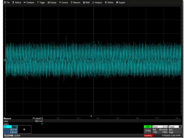
Figure 8: AIF11BAC-01N Ripple and Noise Measurement Vin = 230Vac Load: I o = 10.5A I SB = 0.25A Ch 1: V O
