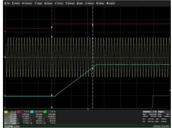
Figure 2: iHP24H3A-S2-00 Turn-on delay via Global inhibit Vin = 380Vac Load: I_O = 12A I_{SB} = 1A Ch 1: AC Mains Ch 2: Global inhibit Ch 3: V_O Ch 4: Global DCOK
