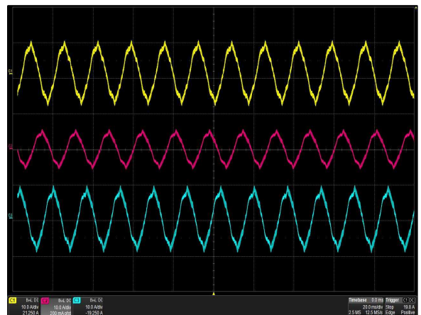
Figure 6: iHP24H3A-S2-00 Input Current Waveform Vin = 380Vac Load: I_O = 12A I_{SB} = 1A Ch 1: Line 1 Ch 2: Line 2 Ch 3: Line 3
