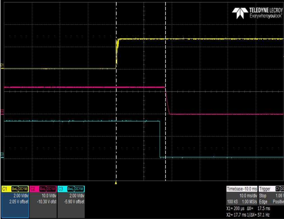
Figure 7: DS495SPE-3 Turn Off Characteristic via PS_ON_L Load: I_O = 41.25A Ch 1: PS_ON_L Ch 2: V_O Ch 3: Pwr_GOOD
