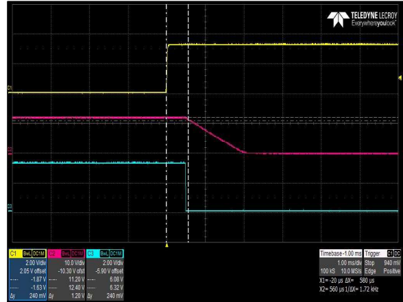
Figure 8: DS495SPE-3 Turn Off Characteristic via PS_KILL_L Load: I_O = 41.25A Ch 1: PS_ON_L Ch 2: V_O Ch 3: Pwr_GOOD
