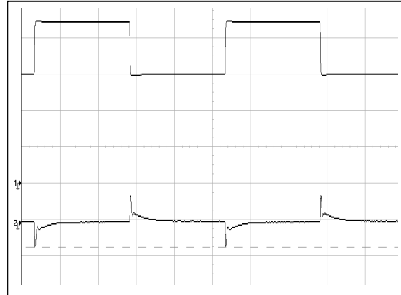
Figure 8: AGF800-48S28-6L Transient Response 50%~75%~50% load change, 0.1A/uS slew rate, Ch 1: Io (5A/div) Ch 2: Vo (500mV/div)
